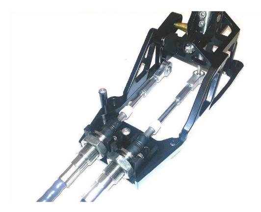
When installing the cables components make sure to apply the plastic caps to all ball end mounts.
