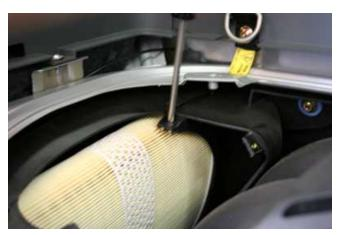
4. Remove the 1, Phillips head screw that attaches the OEM filter to the air box.
