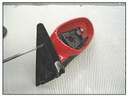
Undo the screws and remove the housing from the arm.
