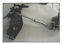
Compress the spring and remove the U-clamp.
