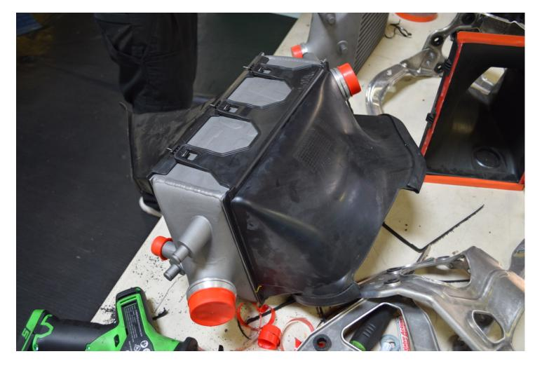
Intercooler assembled and secured. Ready to be installed back into the vehicle.
