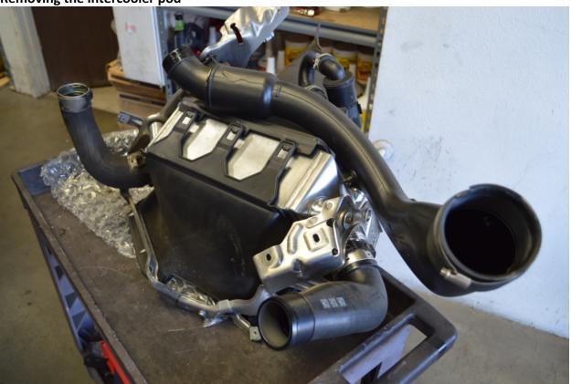
CSF recommends, for easiest installation, to remove the entire intercooler pod – including both intercooler shrouds and all hoses. It is much easier to install a new high performance intercooler if the full pod is out of the vehicle.
