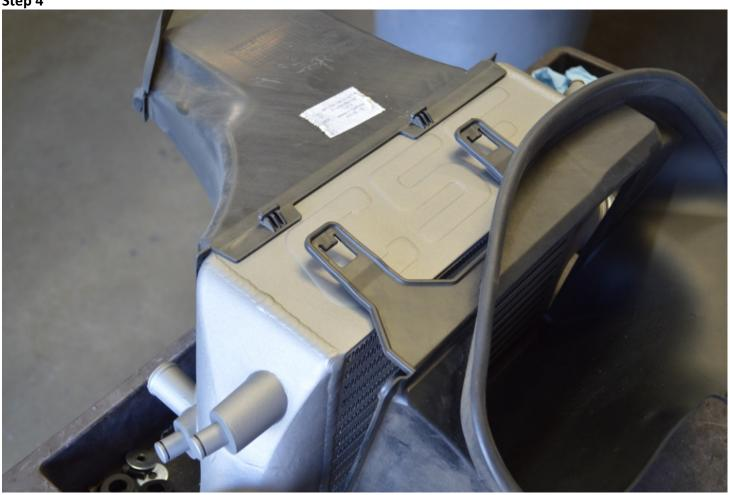
Because of the increased thickness of the core from the OEM 80mm (3.15 inch) to the CSF 115mm (4.52 inches), after trimming the inside of the shroud there will still be a connecting gap of the plastic shroud locking mechanism.
