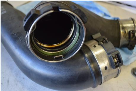
There may be oil that has collected from the turbos in the lower intercooler piping. It is recommended to clean the oil out of these hoses before installing the new intercooler. Please be careful not to disrupt, remove, or tear the sealing O-ring inside the OEM "quick-connect" fitting.
