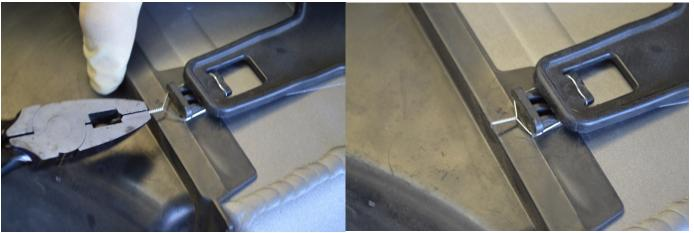
Twist the wire to create tension and a tight seal between the shrouds and the intercooler surface. (you may want to include some simple weather foam stripping between the face of the shroud and intercooler core for optimum airflow through the intercooler core (see picture of 3m tape being applied in step 3).
