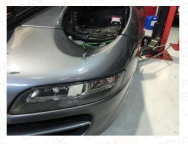
15. Take new lamp and join green wire of mini loom to green loom of headlamp and the same with the black wire.
