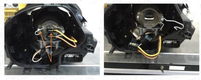
9. Remove 6 screws that hold rear cover on new headlamp then fit bulb. Secure with clip and fit connector.
