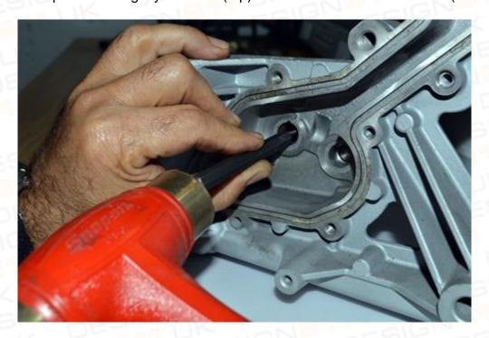
Step 9: Insert new 8MM Drive Key with oil passage slot.
