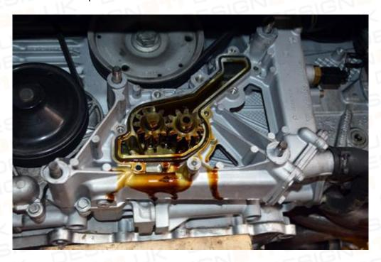
Step 5: Remove the Oil Pump Drive (8MM Allen)
