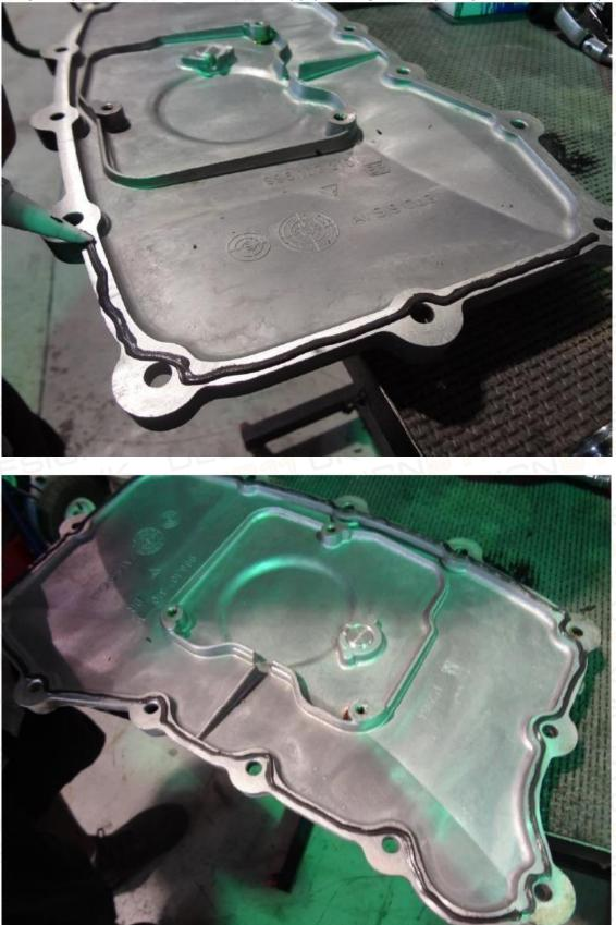
**Step 5:** Using the provided Reinzosil sealant, apply to edge of oil pan (as shown below)
