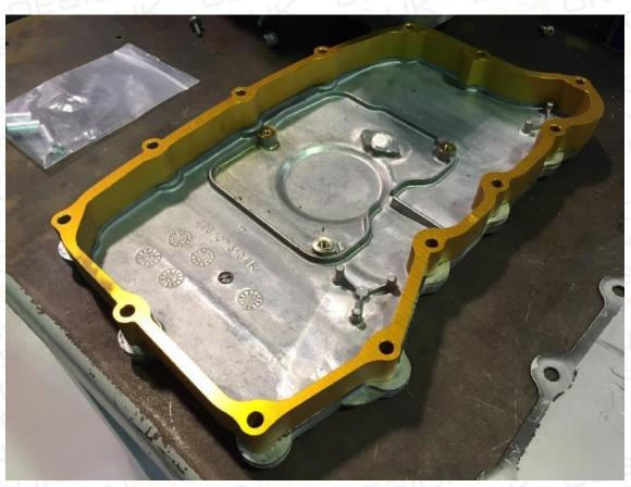
Next, mount the baffle plate to the deep sump extension
