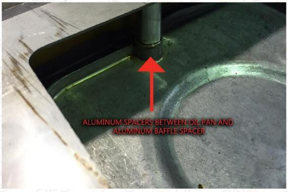
With the baffle in place, align the 3 aluminum 1" spacers between the baffle plate and oil pan.
