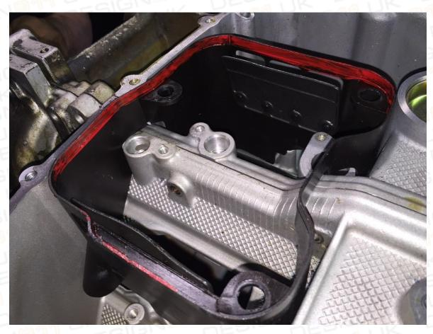
On the same plastic baffle, remove 5mm of the area marked in red in the photo. (shown above and below)
