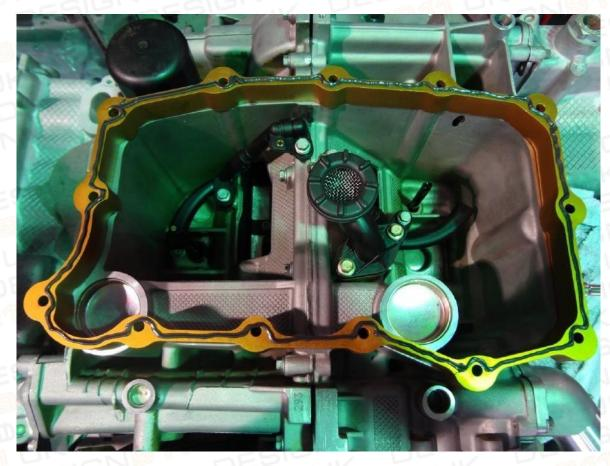
Mount the deep sump extension to the pan. (Note, the photo does not show the pan extension with the sealant. Make sure you have applied the sealant before installing the aluminum baffle on top).
