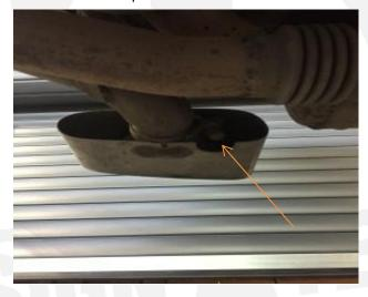
12. Undo the four 17mm headed bolts that hold the clamps between cats and back boxes.
