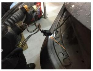
4. Undo the two plastic Scrivets with No 2 Philips screwdriver and remove.
