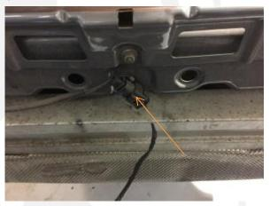
9. Undo the two T30 headed screws that hold the crash bar heat shield to the rear box heat shields (1 each side) and the two 16mm headed bolts that hold crash bar to the car.
