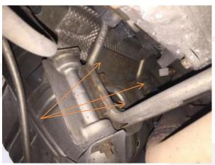
14. On each back box undo and remove the two 13mm headed nuts and bolts that hold the brackets on to the boxes.
