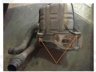
15. Fit Brackets to new exhaust boxes but leave nuts and bolts loose.
