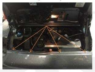
8. Starting with the front corners pull the bumper away from the car. With bumper half off disconect number plate wiring. (there may also bee parking sensor loom if fitted).
