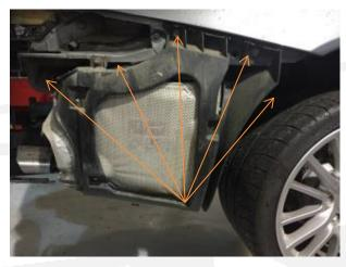
11. If using old tips then undo 13mm nuts that hold tips to back box and remove.
