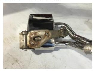
16. Fit clamps to cats (we recommend replacing with new).
