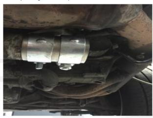
17. Fit new boxes to car, sliding into cat clamp first then installing the three nuts that hold bracket to car.
