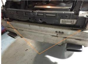
10. Undo the five 10mm headed nuts and bolts that hold back box heat shields to car each side.
