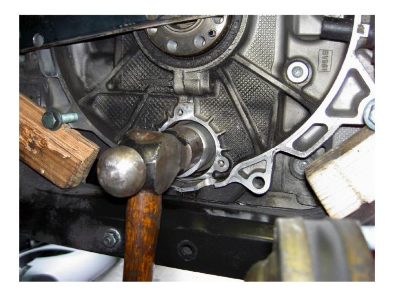
Pull the insertion tool out. The correctly installed bearing should look like this:
