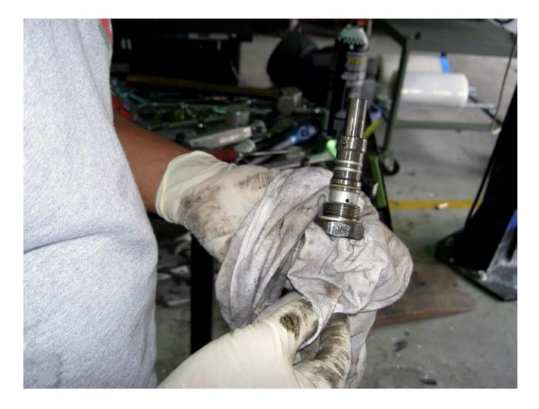
Insert and tighten the chain tensioner.
