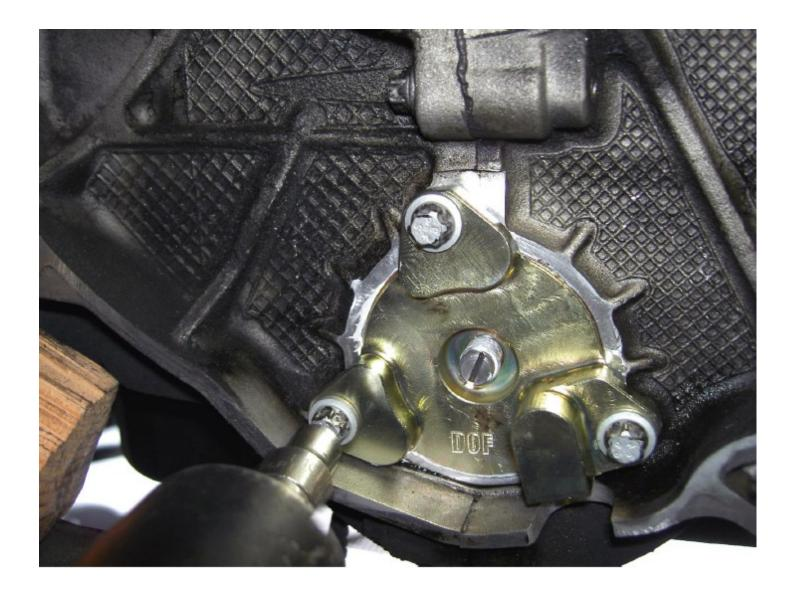
Once al three bolts are completely screwed in and the flange has been seated, tighten to a torque of 10 Nm (7.5 lb-ft or 88.5 lb-in).
