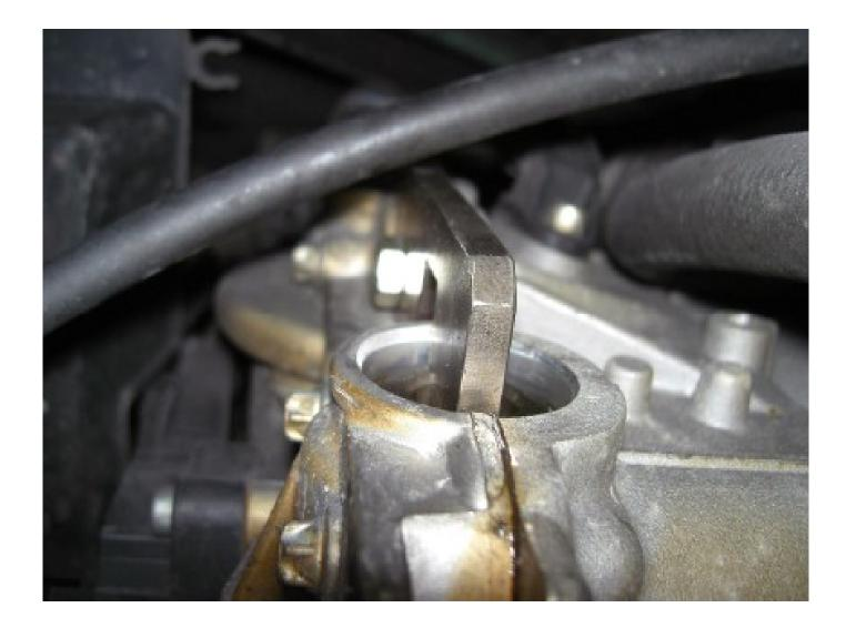
Also, lock the engine's crankshaft to avoid any movement during installation.
