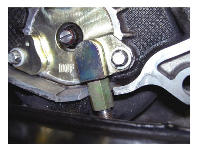
Tighten to a torque of 13 Nm (10 lb-ft or 115 lb-in).
