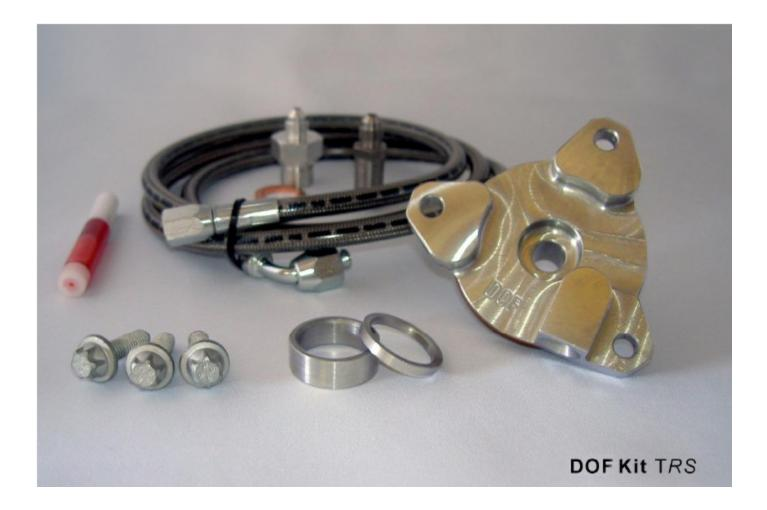
Cars with the double-row bearing use the small spacer (ring) and cars with the single-row bearing use the large spacer (ring).
