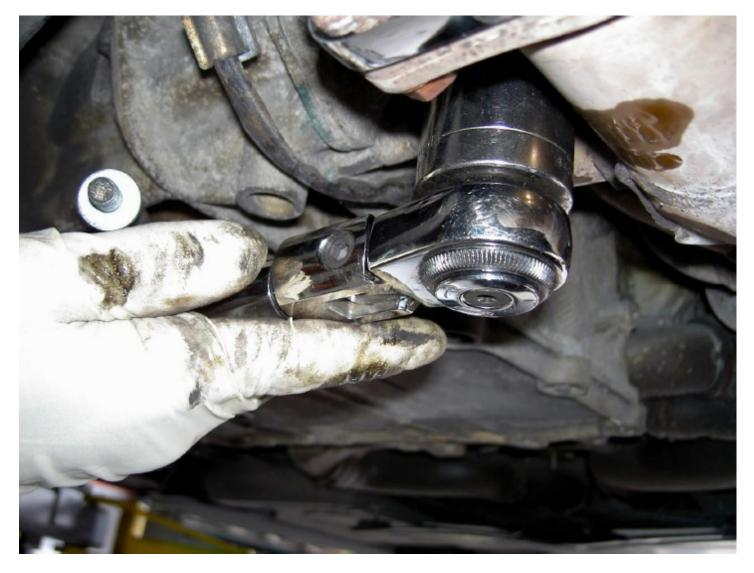
Remove the cam locking key and lightly tap the (supplied) green cam seal in place.
