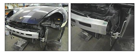
You may also need to bring the front bumper beam forward slighty by using a packer made from metal and londeer bolts
