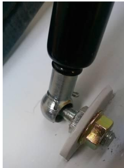
Step 9. Mount the trunklid lifter and fix it with the secure pins
