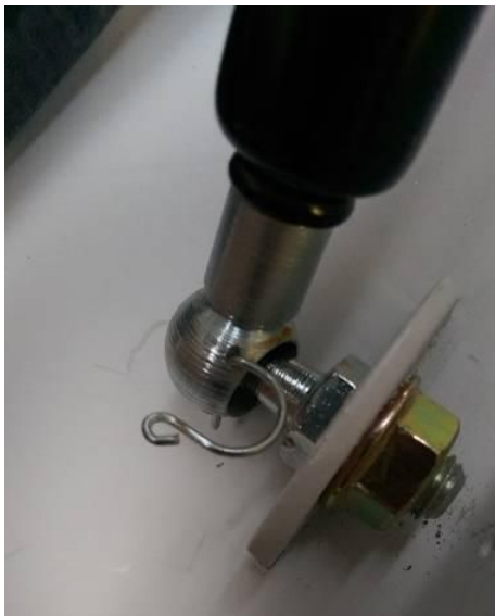
Step 9. Mount the trunklid lifter and fix it with the secure pins
