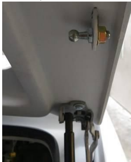
Step 8. Fix the joints for the trunklid lifter on the hardtop and the trunk lid
