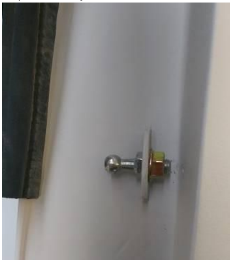
Step 8. Fix the joints for the trunklid lifter on the hardtop and the trunk lid
