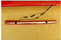
Remove the two screws, withdraw the light module, and unplug the two "banana" connectors by gently pulling them apart. Proceed with changing out the light module as described below.
