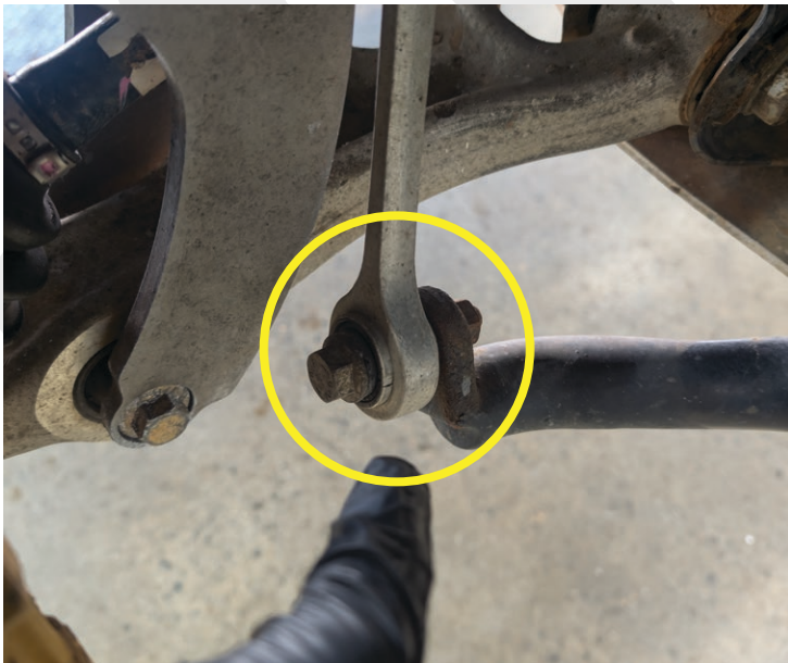
Remove lower sway bar link bolt and nut 18mm
