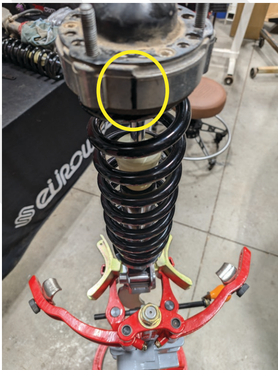
When reinstalling, make sure the top hat aligns with the shock body
