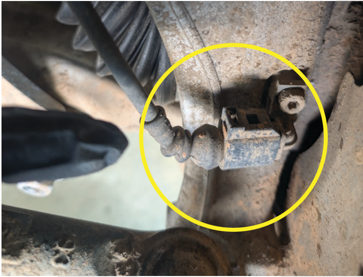
Unplug ABS Sensor. Push the whole harness out the way
