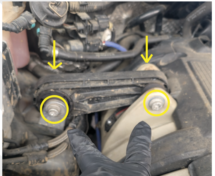
Remove two t50 bolts and two 16mm nuts on the other side
