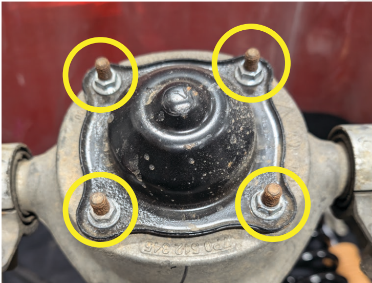
Remove the four top hat cover nuts
