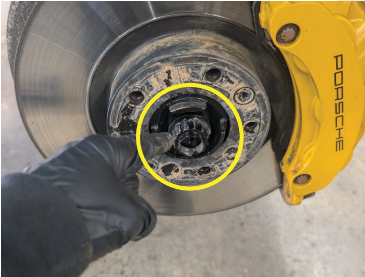
Remove axle nut 32mm
