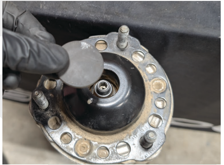
Install rubber seal then install coilovers. This completes the front coilover section and now onto the rear.
