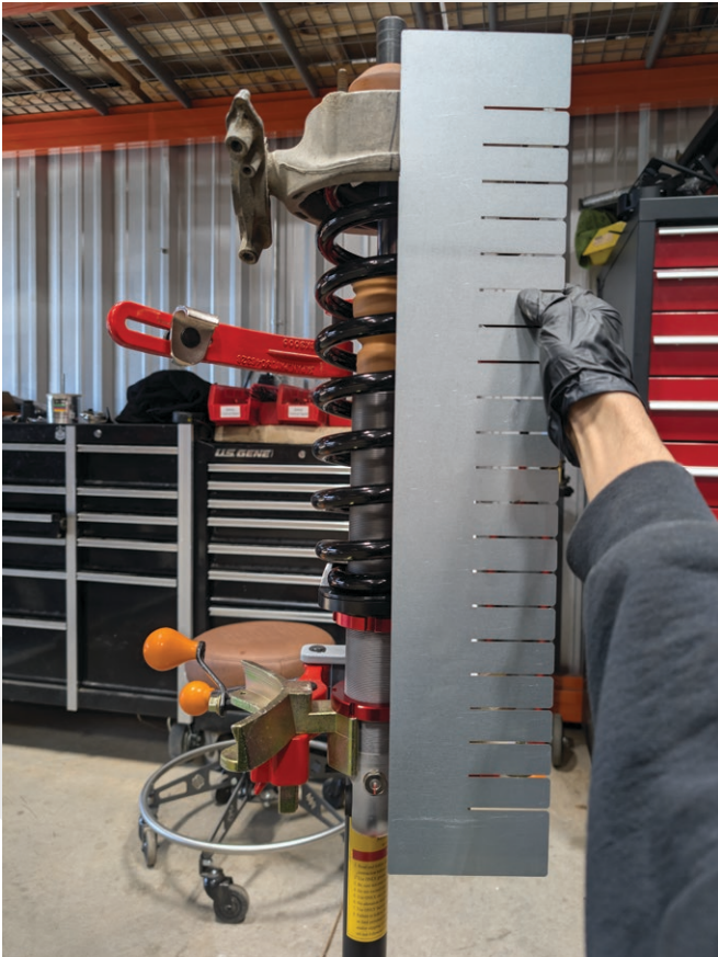
Install top hat and make sure it's aligned with the shock body.
