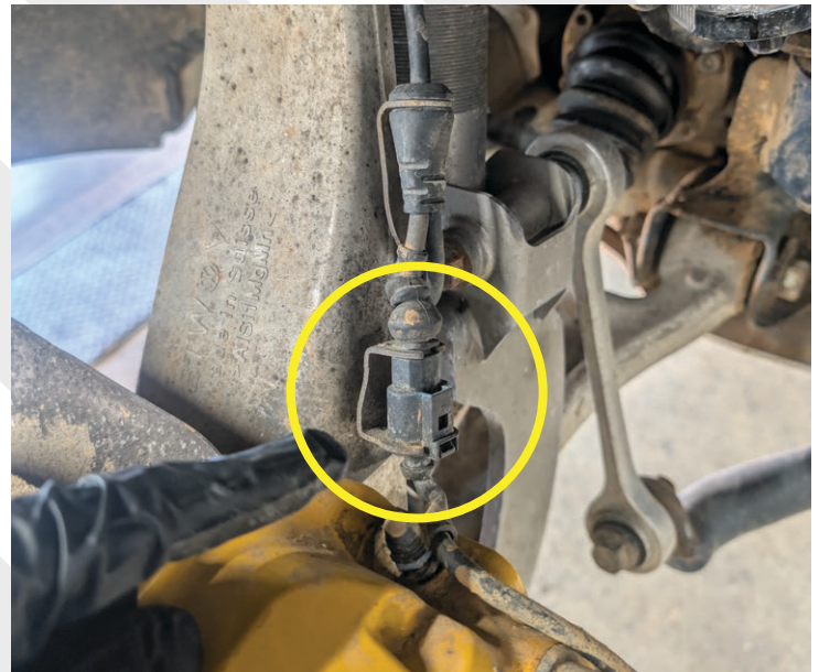
Unplug brake sensor wiring
