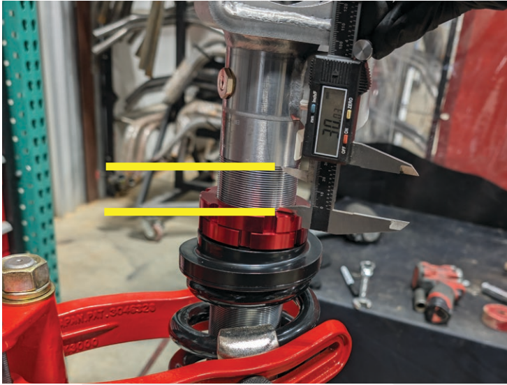
Pre-load coilover to 30mm as shown
