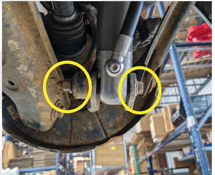
Remove lower shock mount bolts and nuts with a 18mm on both sides.
