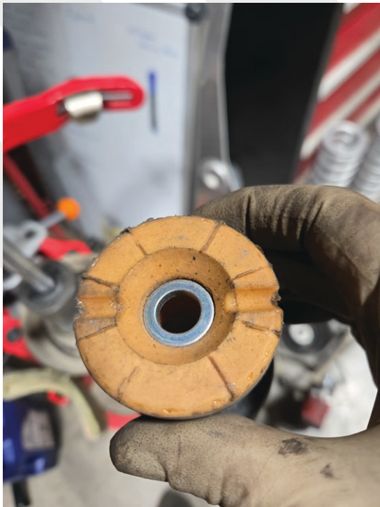
Spacer washer may be stuck in bump stop - make sure to reinstall back in proper order
