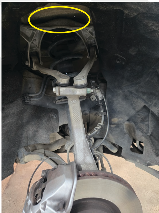
Upper strut mount should be loose at this point
