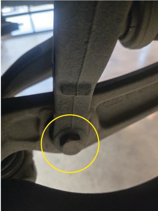
Remove 18mm bolt and nut on both sides
