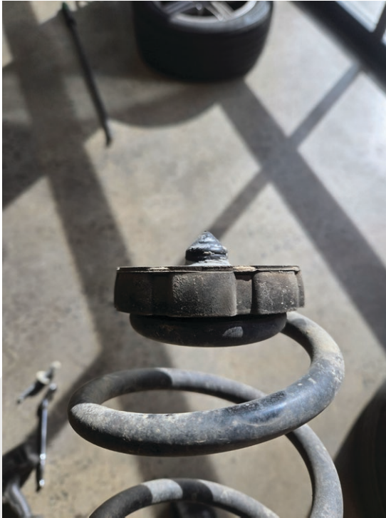
Leave upper isolator installed on coil spring
