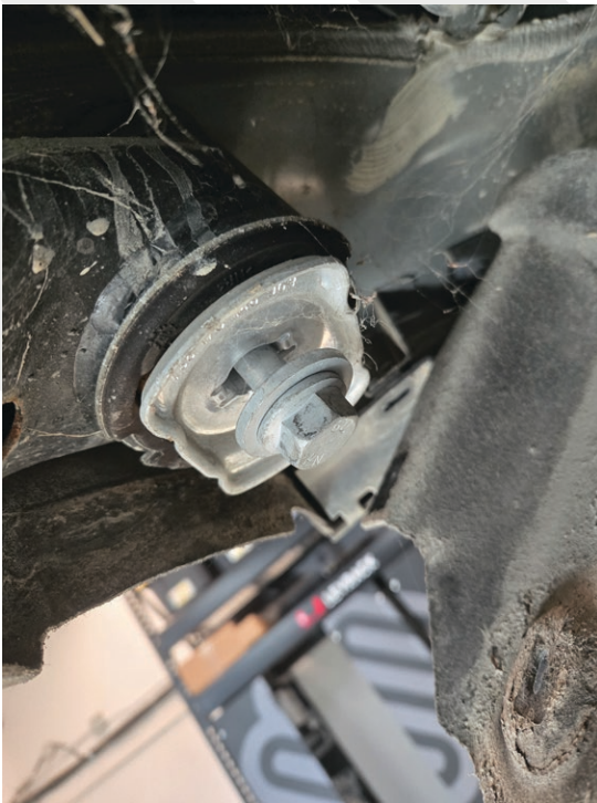
Reinstall subframe bolts - If sway bar link bolt is removed - Now would be the time to reinstall
