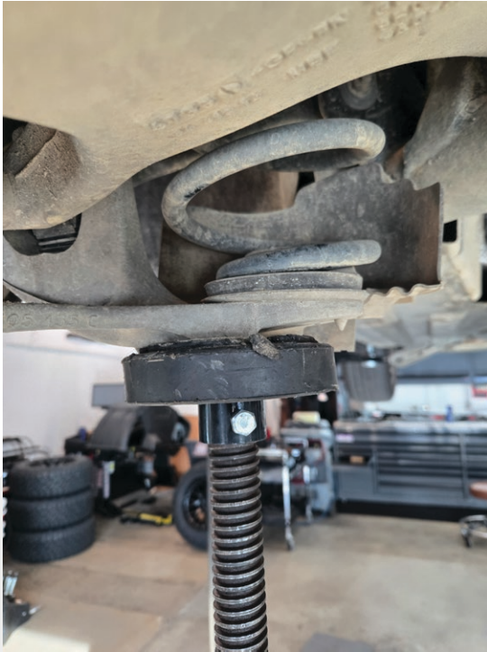
Lower trailing arm to release tension on coil spring and remove spring from vehicle
