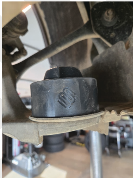
Install rear coil spacer on trailing arm.
