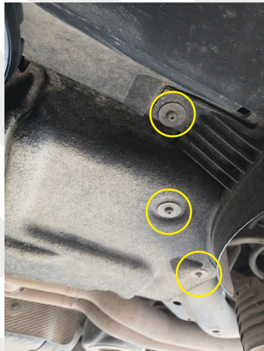
Remove these bolts on both sides to lower underbody cover to allow access to rear subframe bolt.
