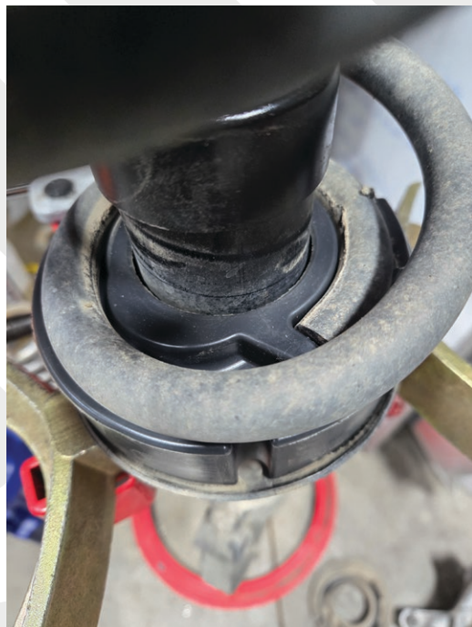
Install coil spring - be mindful of orientation of spacer
