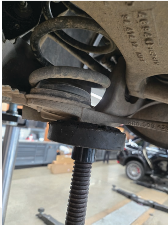
Support rear trailing arm before removing
