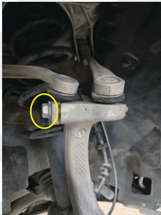
Remove this 16mm pinch bolt and nut to release the upper control arms on both sides
