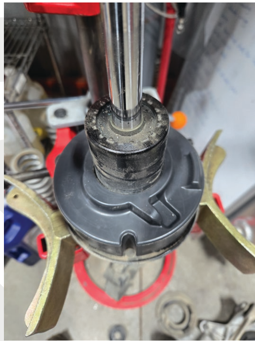
Install front lift spacer on strut
