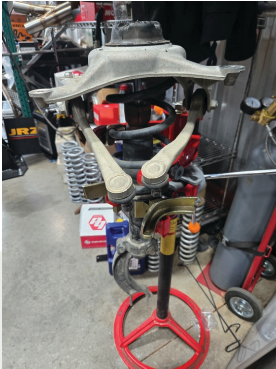
Compress coil spring to remove upper strut nut and remove strut mount assembly
