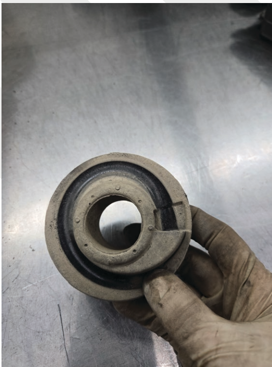
Remove lower coil spring isolator from spring
