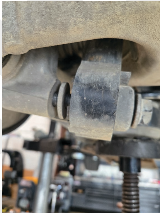
Reinstall shock - Note location of shock bolt washer
