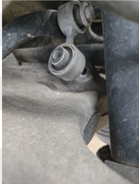
If there's too much tension to remove spring sway bar link bolt can be removed from trailing arm for better access
