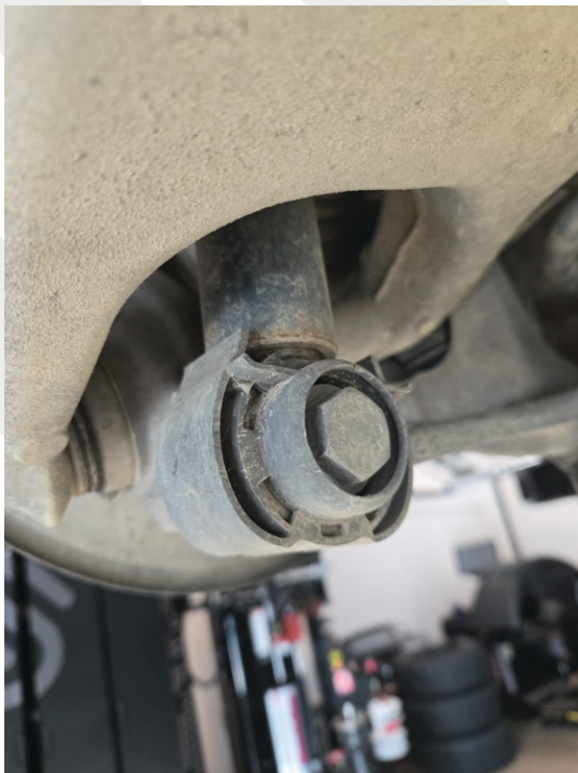
Remove lower shock bolt - Be mindful of washer location between shock and control arm.
