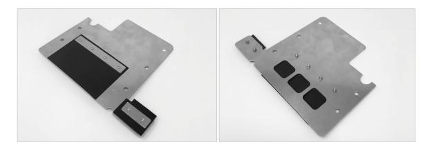
2. Install baffle parts B and D on plate B with six M2.5 bolts, nuts and Loctite as shown.
